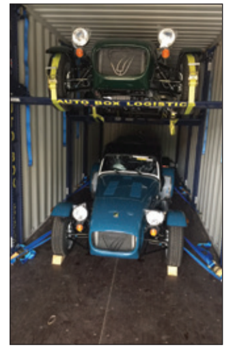
Demand for containerised shipments includes high-value vintage/veteran autos, such as these Caterham Super 7s, secured with TRI's R-Rak
