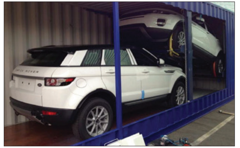
The WMG software increases the racking potential in a 40ft high cube container from three to four vehicles
