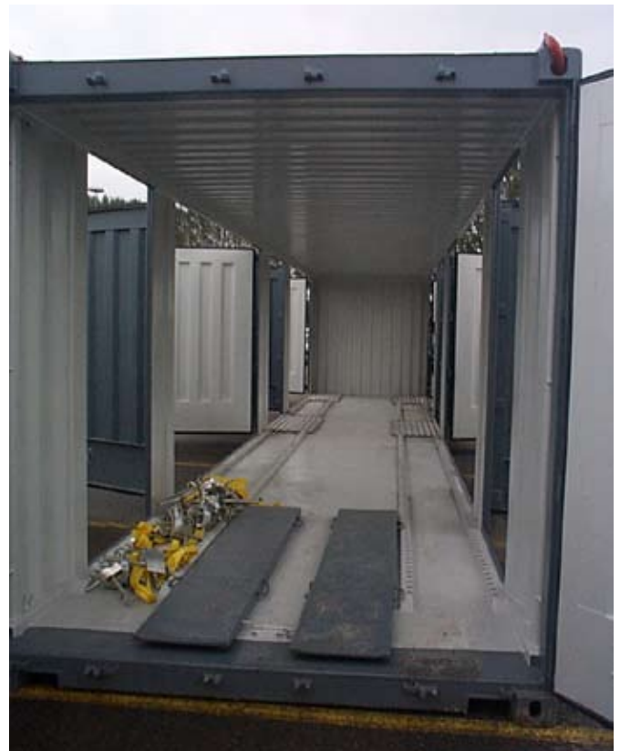
Damco's 20ft containers have four doors as standard, to give access to the vehicles loaded inside without running the risk of damaging them
