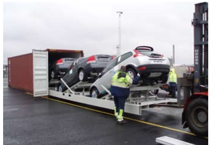
Containers for cars can be divided between those loaded inside the container and those pre-loaded on cassettes outside
